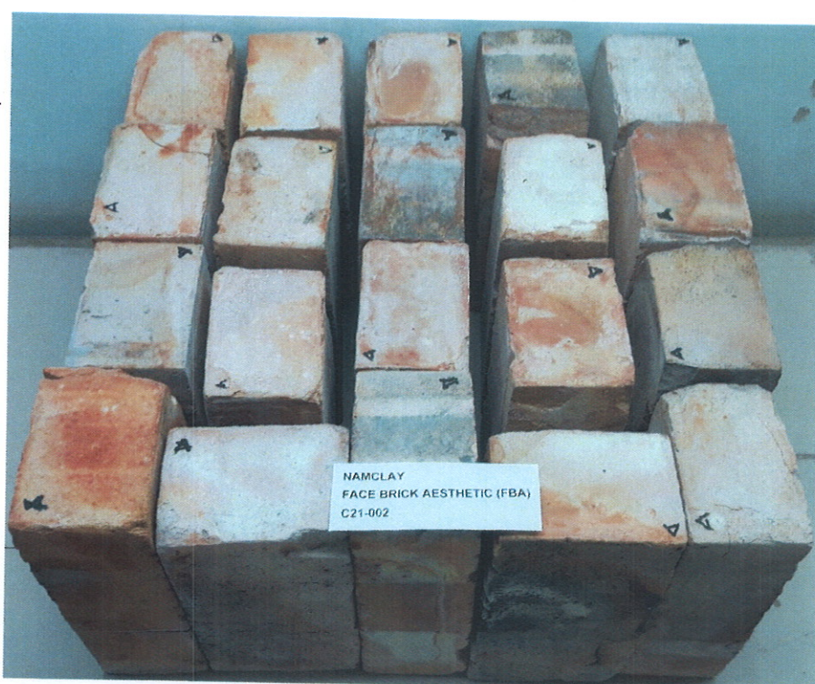
Figure 3.5.1: Samples after efflorescence testing
